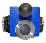
The pencil tip protrudes about 5 mm out of the holder block. Place the **TriForcePencil** carefully on the sample, set up first with the wheels and after then with the pencil tip. Lower the device slowly by index finger under the round knob of the lift arm. The hubs of the wheels are held with the thumb and forefinger and the instrument is moved over the specimen in the direction the pencil point shows at a speed of about 10 cm/s.
