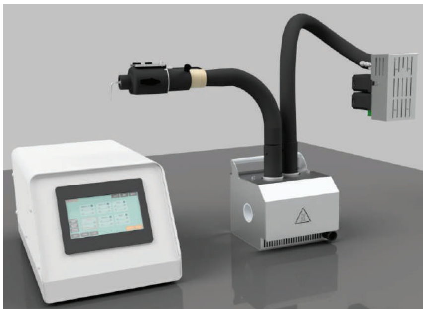
Figure. Example of TG-IR-GC/MS with digital controller
