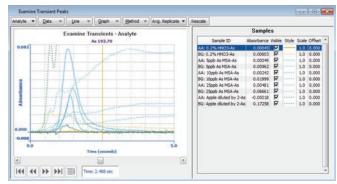
Examine Transient Peaks Window allows you to view the effects of changing various analytical parameters for accelerated method development.
