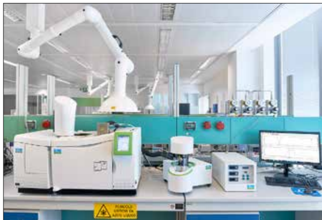
Figure 1. TG-GC/MS (Clarus SQ 8 GC/MS, TL8500, TGA 8000).
