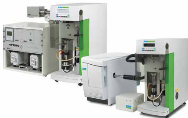
Figure 1. Pyris 1 TGA is shown interfaced to a HPR-20M (left) and a TurboMass 600 MS (right).
