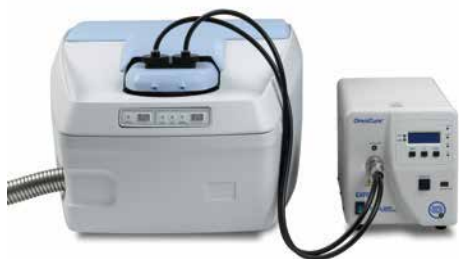
Figure 1. Picture of DSC 8000/8500 with the OmniCure® 2000 UV accessory showing sample and reference light guides.
