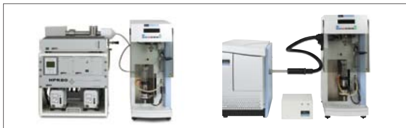
Figure 1. Pyris 1 TGA is shown interfaced to a HPR-20 MS (left) and a Clarus 600 MS (right).
