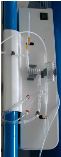
In line UV digester for Total Phosphorous, Total Nitrogen etc., dedicated lamp for Total Cyanides
