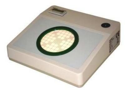
The new Astor 20 Colony Counter is very easy to use. Thanks to its Petri dish holder, back-lit and sensitive to pressure, the enumeration of the microbial grown colonies on the agar surface can be performed by a simple and common marker. The Petri dish holder is back-lit by LED's: this new technology grants a better light diffusion, a greater reliability and a minimum power consumption (2 W, as a total).
