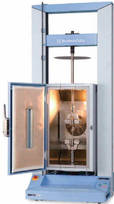
AGS-10kNXD + Screw Type Flat Grips + Compact Thermostatic Chamber TCE series
