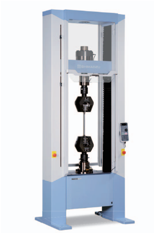
AGS-300kNX + 300kN Non-Shift Wedge Type Grips
